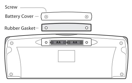
FIGURE 4. Keyboard Battery Installation
